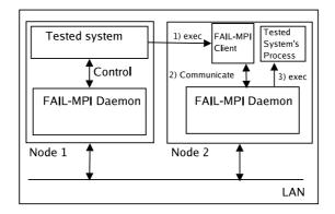
Figure 3: FAIL-MPI integration scheme
