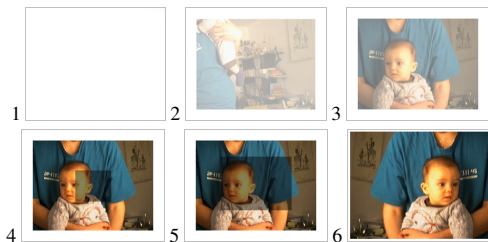
Figure 8: Transitions between the sleep mode (1), the mirror mode (2 to 5) and the picture transmission mode (6).
