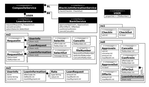
Fig. 2. xLoan Example – Data and Service Architecture
