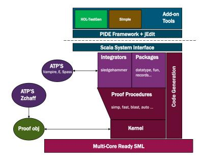
Figure 2.1: The diagram shows the different layers like execution environment, kernel, tactical level and proof-procedures, component level (providing external prover integration like Z3, specification components, and facilities like the code generator, the Scala API to the system bridging to the JVM-World, and the Prover-IDE (PIDE) layer allowing for asynchronous proof and document checking.
