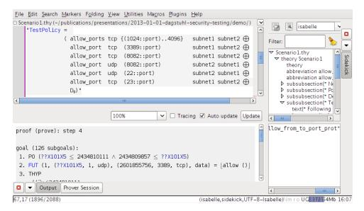
Figure 3.1: An Isabelle session showing the jEdit client as Isabelle Interface. The upper-left sub-window allows one to interactively step through a test theory comprising test specifications while the lower-left sub-window shows the corresponding system state of the spot marked in blue in the upper window.
