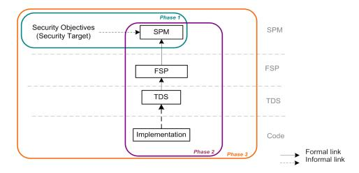
Figure 3.2: Refinement steps for a formal development approach compliant to CC
